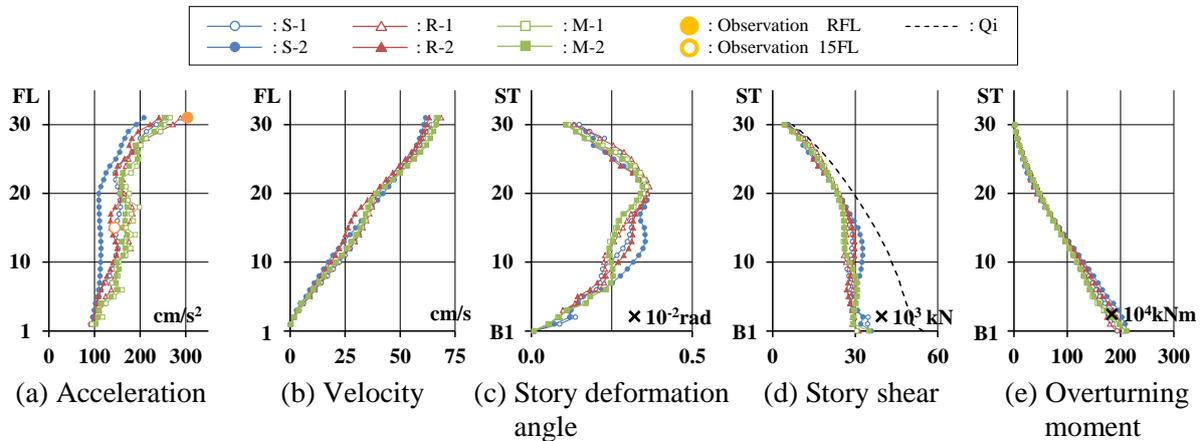
Figure 9. Comparison of maximum responses due to different damping models (Y direction)
