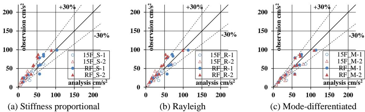
Figure 5. Comparison of maximum response acceleration from analysis results and observation records (X direction)
