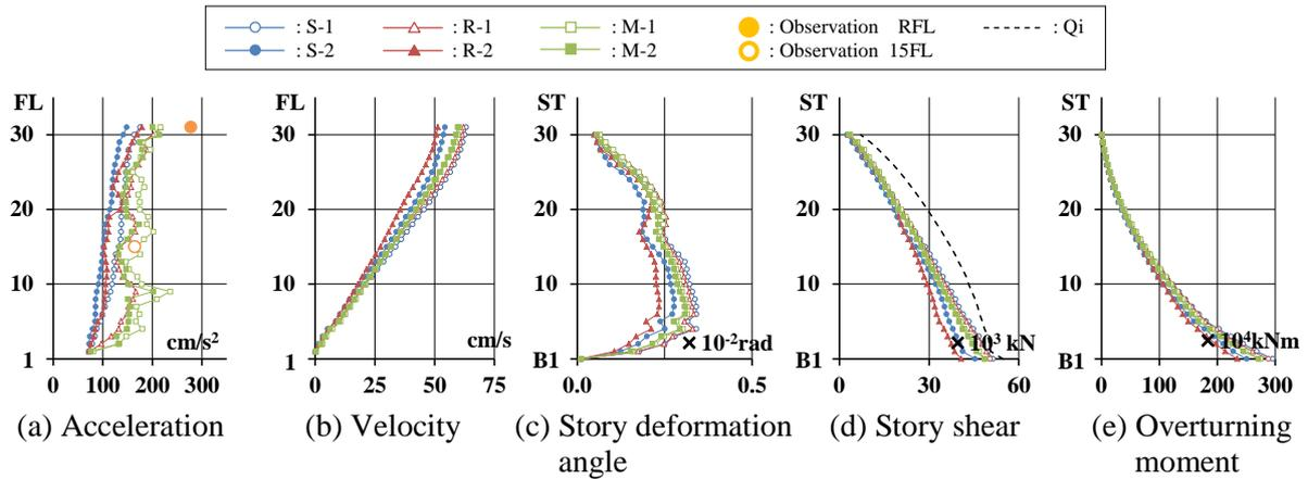
Figure 8. Comparison of maximum responses due to different damping models (X direction)
