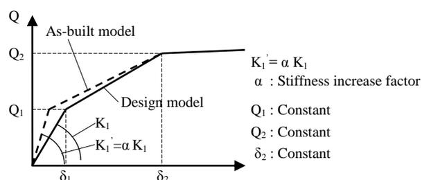
Figure 2. Consideration method of the stiffness increase factor on the skeleton curve
