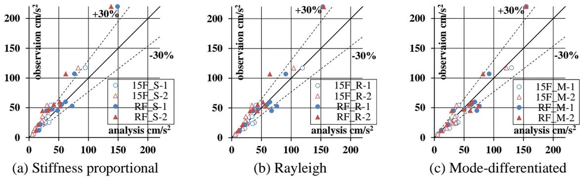
Figure 6. Comparison of maximum response acceleration from analysis results and observation records (Y direction)
