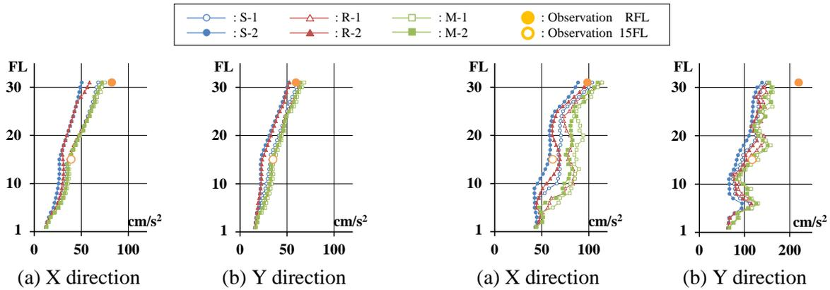
Figure 3. Maximum response acceleration (observed wave record No.4)
